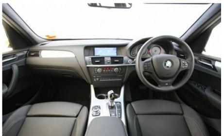
The Navigation System has a high-resolution 8.8" Control Display, iDrive Controller, including one-touch keys and favourite buttons, 2D/3D display, split screen function, 20GB hard drive for storage of audio files, satellite images and electronic owners handbook.
