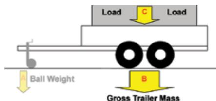
**Gross Trailer Mass (GTM)** – the mass transmitted to the ground through the axle(s) of a trailer when the trailer is loaded.
