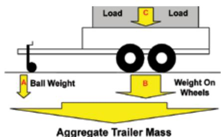
**Aggregate Trailer Mass (ATM)** – the total laden mass of the trailer.
