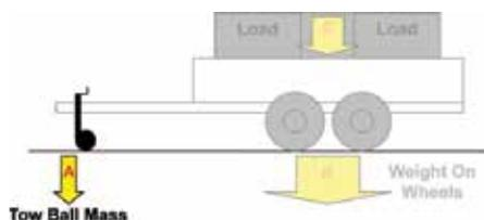
**B Weight on Wheels** – the vertical down force transmitted to the ground through the trailer axle(s) excluding the load
