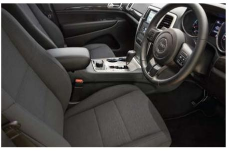
full-length side-curtain air bags, seat-mounted side thorax air bags, standard driver inflatable knee bolster and active head restraints that deploy in the event of a rear collision.
