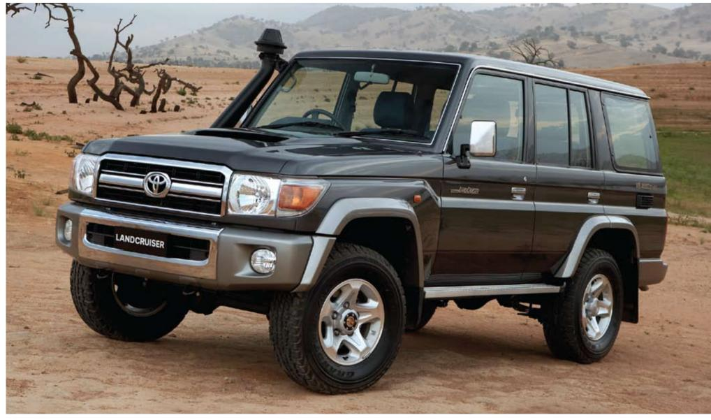
Toyota's indestructible Landcruiser 76 Series Workmate Wagon is one of the few 4WD's that I would confidently drive from the showroom to the centre of Australia. The Workmate has stayed with the traditional construction of ladder frame chassis and live axles front and rear and the test vehicle was also fitted with factory option front and rear diff locks.
